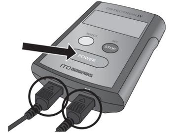
Two probe leads inserted
